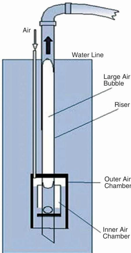
Fig. 2: Schematic of a Geyser pump
