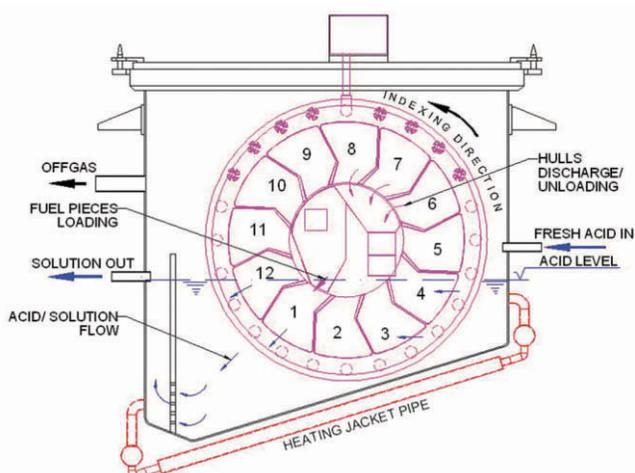
Fig.1: Schematic of a Continuous Rotary Dissolver
